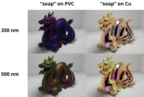
Figure 6: Soap ( $\eta_2 \approx 1.33$ ) films on PVC ( $\eta_3 \approx 1.54$ ) and Copper with film thicknesses given on the left.
